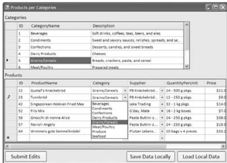
FIGURE 18.18 Displaying product categories and suppliers in a ComboBox control on the DataGridView control
