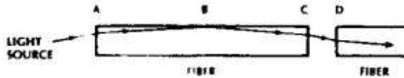
Figure 3-19 Reflecting surfaces in a fiber system. Light rays are reflected at the input (A), at the core interface (B), and at the boundaries of an air gap formed at a connector or splice (C or D).
